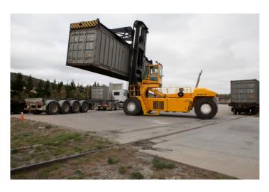
'Increasing the payload per container was easy. This was because the original containers were modified through the fitment of a false wall which limited the cubic area occupied by the compacted waste. This wall was originally included to ensure total payload and its distribution within the container to comply with triaxle group and gross mass limits. All we had to do was remove it to gain the additional payload we wanted using the quad axle grouping.'
