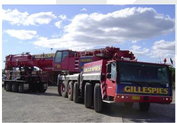
'The industry in NSW wanted the 3.1 metres width adopted as a maximum allowable standard for mobile cranes, to ensure consistency with access conditions in Victoria and Queensland. A compromise was reached where the RTA agreed to allow the operation of mobile cranes up to a maximum width of 2.9 metres under the MCCBS.
