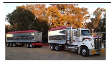
Mr Cook said that, 'Quad dogs operating under the IAP are able to do so at a Gross Vehicle Mass (GVM) of 57.5 tonnes while quin dogs can operate at 63 tonnes GVM. In terms of payload this works out to 40 tonnes on the quad dog unit and 44 tonnes on the quin dog unit.'
