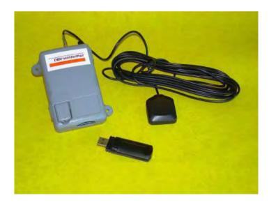
Figure 28: On-Board Equipment used by the DBV-Winterthur insurance company in Germany
