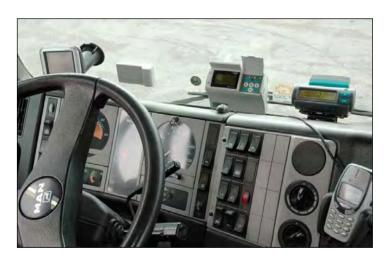
Figure 20: For heavy vehicles interoperability of charging systems becomes a necessity Picture taken from a truck at a Swiss/German border crossing with the following equipment on the windscreen: (from left to right) navigation system, Austrian DSRC-based OBU, Swiss Tachograph-based OBU, German GPS-based OBU.
