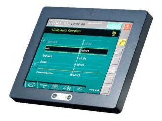
Figure 4: Mobile touch-terminal for driver
