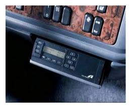
Figure 7: German radio-slot sized Toll Collect OBU
