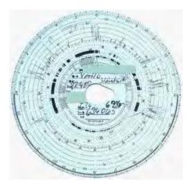
Figure 9: Disk of an Analogue Tachograph
